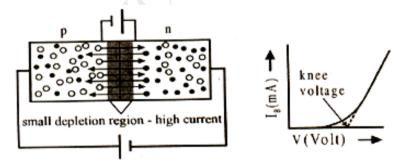
The P-N junction is said to be forward biased when the P-side of the junction is connected to the positive terminal and the N-side is connected to the negative terminal of the external source of emf.
