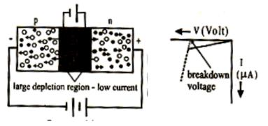
The P-N junction is said to be reverse biased when the P-side of the junction is connected to the negative terminal and the N-side is connected to the positive terminal of the external source of emf.
