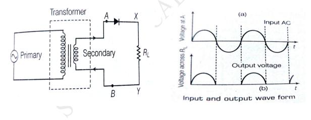
A half wave rectifier is one in which rectification is done for only one half cycle of input AC.
