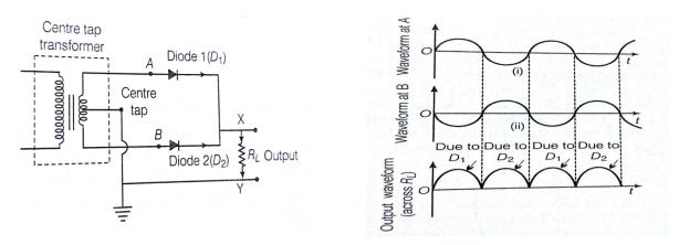
A full wave rectifier is one in which rectification is done for the complete (both) cycle of input Ac.
