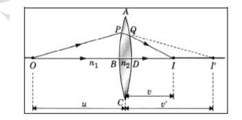
A ray OB incident along the principal axis proceeds undeviated. Another paraxial ray OP after refraction emerges along QI.
