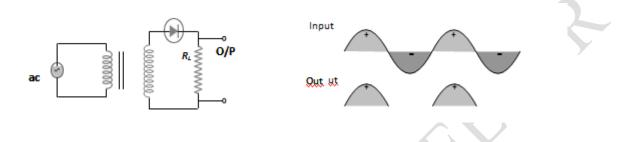
The process of conversion of AC into Pulsating DC is called rectification. **Working:**
