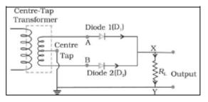
• The full wave rectifier circuit is as shown in the figure
