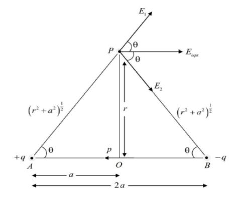
Electric field intensity at P due to the charge +q is
