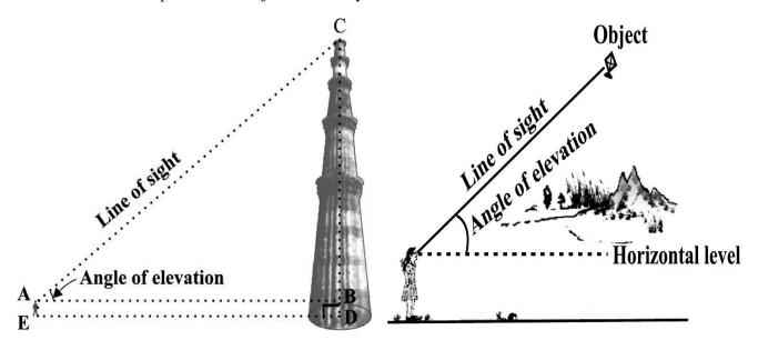
The **angle of elevation** of the point viewed is the angle formed by the line of sight with the horizontal when the point being viewed is above the horizontal level, i.e., the case when we raise our head to look at the object
