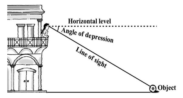
The angles of depression of the top and the bottom of an 8 m tall building from the top of a multi-storeyed building are  $30^{\circ}$  and  $45^{\circ}$ , respectively. Find the height of the multi-storeyed building and the distance between the two buildings.
