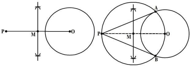
Draw a circle of radius 3 cm from a point 7cm away from its centre. Construct a pair of tangents to the circle and measure their lengths.
